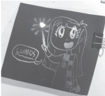
In the picture to the left, a tiny LED light becomes the focal point of a scratch art drawing. This was one of the STEAM activities where kids built the circuit that powers the light using copper foil tape and a lithium coin battery.
